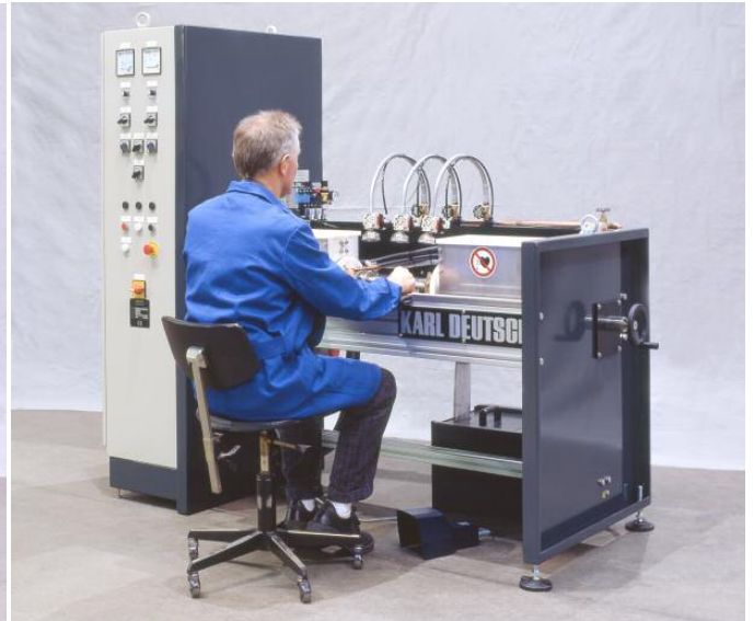
Fig 1. General view of the inspection system including the electric cabinet, the foot-switch for initiating the inspection and the container for the testing agent. The crank (right) moves the yokes. Right photo: place of work with sitting position.
