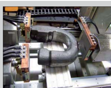
Test machine with moving coil and three current contacts for magnetization of large hooks
