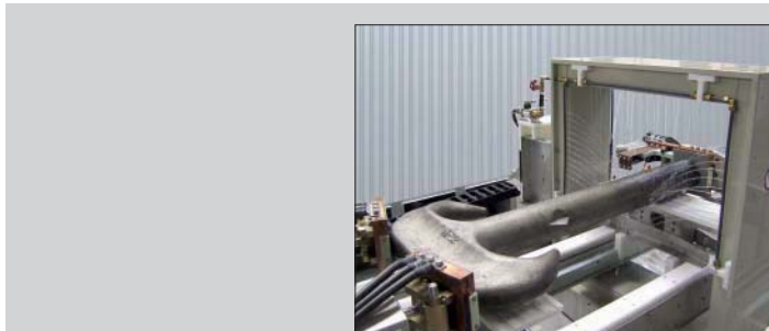
Test machine with moving coil and three current contacts for magnetization of large hooks
