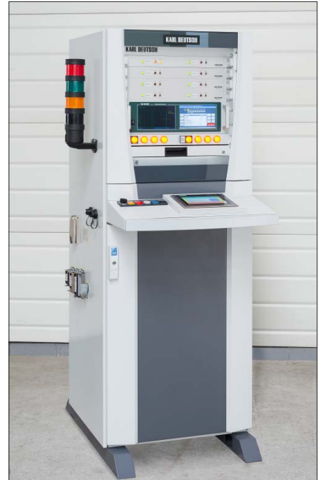
38 HU switching cabinet with operating panel and PLC
