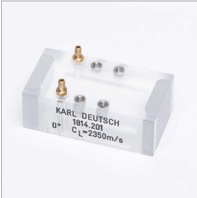
Plane delay 1814.201 with water irrigation
