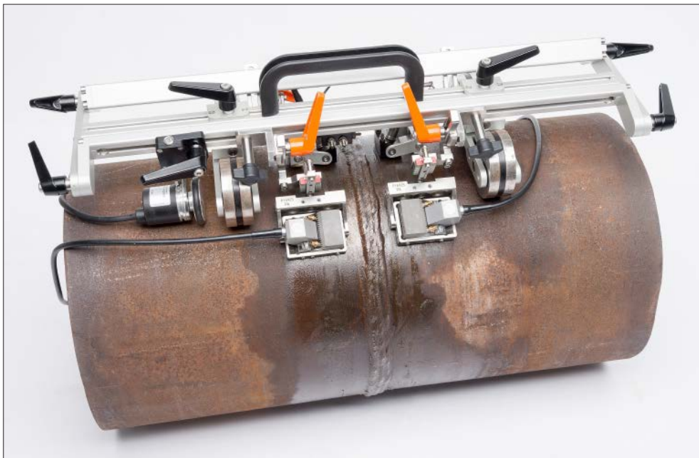
Example of a scanner for manual testing of circumferential tube welds with position encoder and suspensions for 2 phased array probes and 2 TOFD probes
